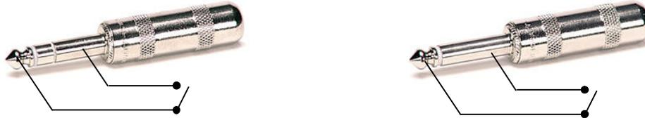
Foot switch plugs showing tip/sleeve wiring for Session Controller operation.
