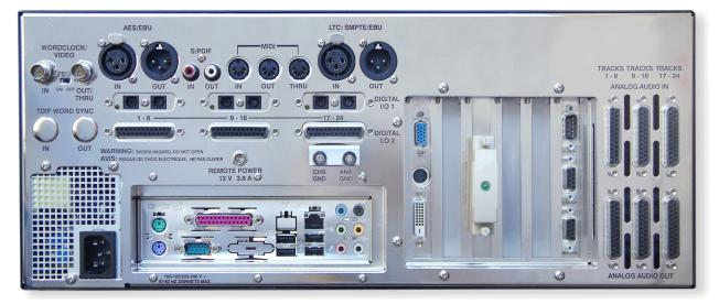
RADAR Rear Panel Labeling (unit shown with optional multi-channel AES/EBU, ADAT and analogue I/O boards)
