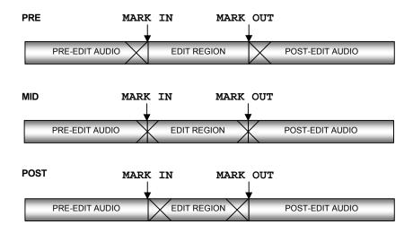
Example: Sometimes when doing an erase with the crossfade set to MID, the mark in point would have a tiny slice of audio waveform after it, which represented the last half of the MID crossfade. This can now be avoided by setting an erase edit to PRE.
