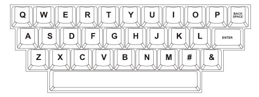
These keys are used to enter names and other information into RADAR®24. They are also used as shortcuts in both transport and menu mode.
