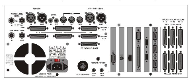
Diagram 1.1 RADAR<sup>a</sup>24 Rear Panel Labeling (unit shown with optional multi-channel AES/EBU, TDIF and analog I/O boards)
