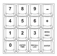
The numeric keypad is used to enter times and other values into RADAR®24. It is also used for recalling single digit locate points 0 - 9.
