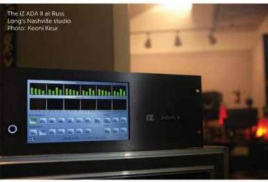
"It comes with either iZ's Classic 96 or Ultra Nyquist converter technology, both of which are identical to those offered in iZ's latest generation RADAR 6." Russ Long
