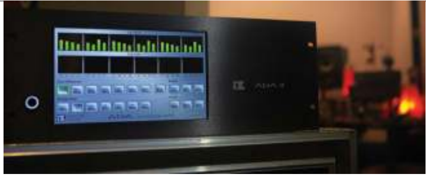
The ADA II's LCD provides access to seven user screens: Main, Setup, Route, Meters, System Configuration, About and Debug.
