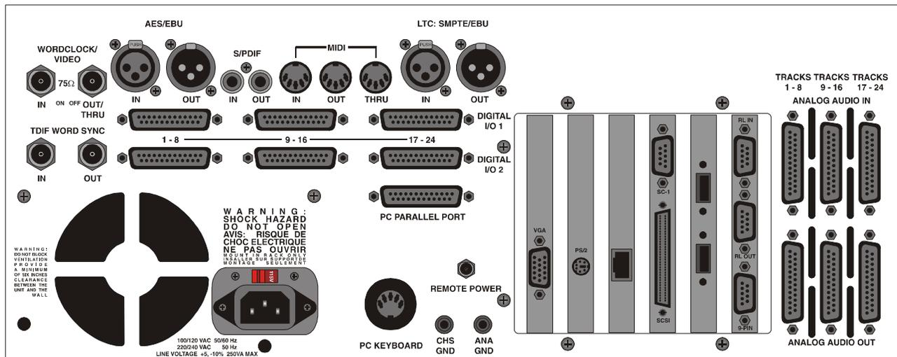
**Diagram 1.1 RADAR<sup>®</sup>24 Rear Panel Labeling** (unit shown with optional multi-channel AES/EBU, TDIF and analog I/O boards)
