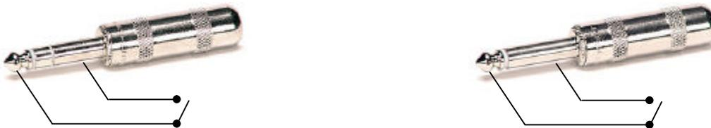
DIAGRAM 1.0 Foot switch plugs showing wiring for Session Controller operation.
