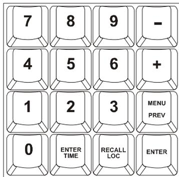
The numeric keypad is used to enter times and other values into RADAR<sup>®</sup>24. It is also used for recalling single digit locate points 0 - 9.
