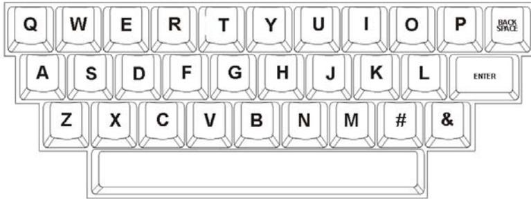
These keys are used to enter names and other information into RADAR. They are also used as shortcuts in both transport and menu mode.
