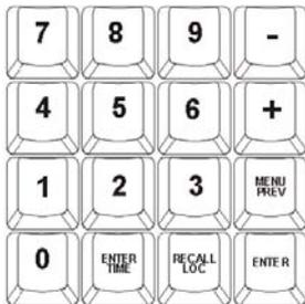
The numeric keypad is used to enter times and other values into RADAR. It is also used for recalling single digit locate points 0 - 9.
