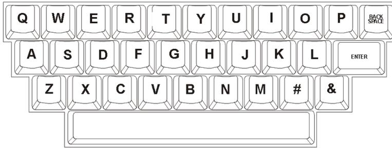
These keys are used to enter names and other information into RADAR®. They are also used as shortcuts in both transport and menu mode.
