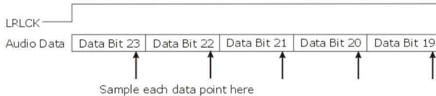
The Audio Framer has no way of knowing that the LRCLK and audio data are not properly aligned. It ends up sampling each audio bit near the end of the bit, rather than in the middle. If there is any jitter on the clock, this could result in sampling a bit at a bit boundary. This will result in clicks and pops in the audio.
