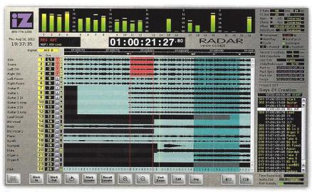
Far more than a simple hard-disk recorder, the RADAR 6 allows quite sophisticated editing of multitrack recordings.
