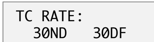
All Time Code rates are available - use the left/right cursor keys to select between 24 fps, 25fps, 30ND (non-drop frame), Select the desired format using the cursor keys, then press ENTER. The TC Format setting will be maintained until changed.
